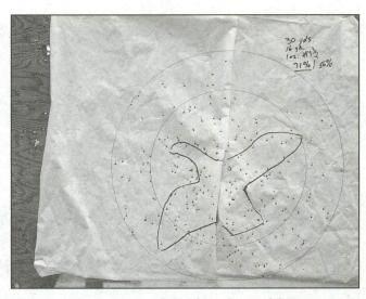
Pattern with one ounce of shot from the Model 12 16-gauge with a 2 9/16-inch chamber.
