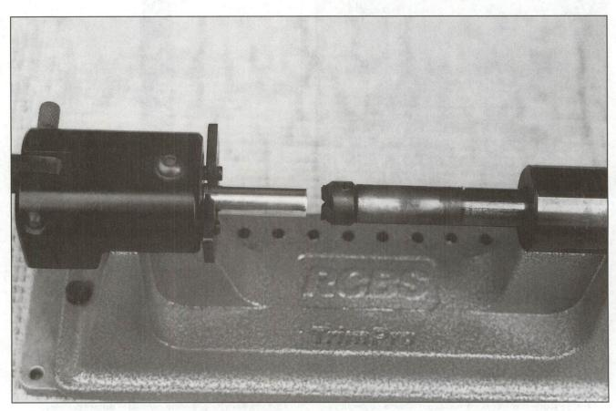
Trimming revolver brass to a uniform length is essential to fine accuracy.
