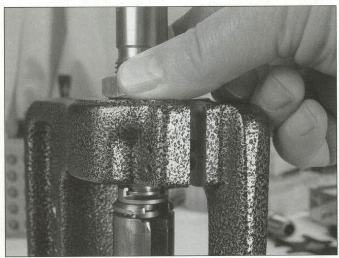
With our bullet seated to the proper depth, the die is locked down with a cartridge in the die, ensuring proper alignment. The same procedure should be used for all die adjustments.
