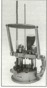
The tall thin tube in the center rear of this progressive reloading press is filled with a stack of primers. If the feeding mechanism jams, the stack can explode if you do not clear it properly. If a jam occurs, read the manual, and if in doubt, call the manufacturer for assistance.
