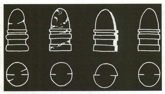
ter filled out than the other. These bullets, along with the sprues, are returned to the melt pot. Expect quite a few of these in the beginning. A good bullet will be evenly filled out everywhere. Corners on drive bands will be square and the bands will be of even width all round. By rolling a bullet across a flat surface irregularities in band width may be easily seen. Discard all those that are noticeably uneven.
