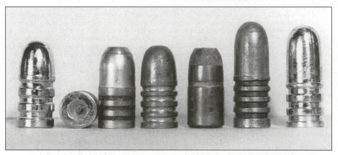
Soft alloy bullets of lead and tin (the shiny ones on the ends) will yield lower pressures than harder alloy bullets. Jacketed bullets (third from right) create significantly higher pressures, as do heavier bullets.
