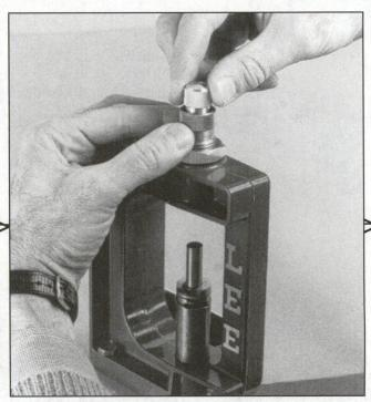
Step 13 - Bullet Seating (B): The knurled adjusting screw controls the bullet seating depth. Usually, seating to the same depth as a factory round works well. If you want a crimp, be sure the bullet cannelure is almost completely inside the case mouth. Screw the die in just enough to apply a good crimp. A little trial and error work is needed here.
