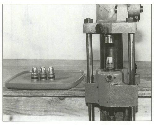
A bullet pops up after having been lubricated on a SAECO machine. A solid mounting is needed to keep the machine from lifting off the bench top. Proper die adjustment is necessary to keep lubricant from squirting over the bullet nose. The small amount seen here can easily be wiped off.
