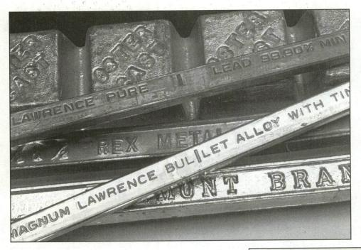
Block lead and tin, as well as pre-mixed alloys, ensure purity in the metal alloy. Many scrap alloys, however, may be used to make good bullets, including wheelweights, lead plumbing pipe and lead cable sheathing. Scrap 22 rimfire bullets recovered from indoor shooting ranges can also be a viable source.
