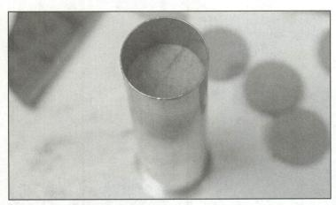
45-70 Govt. case loaded with 60 grains of Goex Cartridge and a fiber wad atop the charge. The thin card wad protects the bullet base but may not be necessary for hunting loads.
