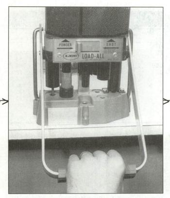
Step 2 - Priming: Place a primer in the priming pocket at Station 2. Move the shell onto Station 2 and pull down the handle. The sizing die will automatically be pushed off the shell at this station. Remove it completely.
