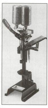
The MEC Steelmaster single-stage press comes automatically set up for steel reloading. It is available to load from 2-3/4" 12- gauge through 3-1/2" 10-gauge, plus can also load lead shot simply by changing out the transport bar.
