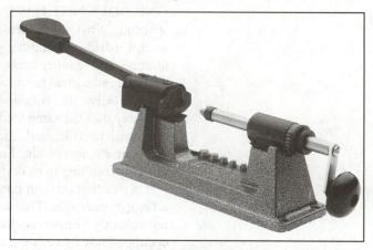
A case trimmer, such as this RCBS model, should be in the equipment inventory of every handloader, particularly those who load high-intensity cartridges like many of the 22 center-fires used for varmint work.
