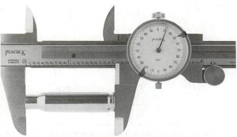
Case length should be checked after sizing and neck expanding.
