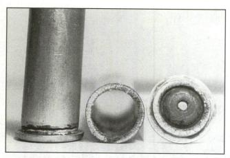
The REM-UMC case on the left suffered near total separation due to mercury contamination. This same factor caused the one on the right to pull apart in the resizing die.
