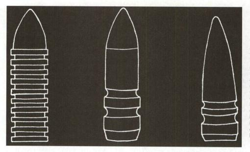
The best rifle accuracy with a cast alloy bullet is with one that has a short ogive. The bullet on the left has many lubricant grooves and will shoot well in multi-groove and shallow-groove barrels owing to good bore contact over most of its length. The center bullet is a "bore-riding" type also with a short ogive. The right bullet is of a long-ogive design. Difficulty in getting such a bullet properly seated in the case makes it a poor shooter.
