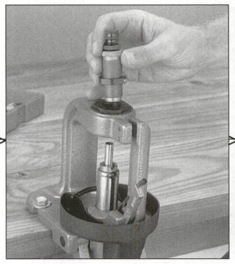
Step 8 - Case Mouth Expansion: This step applies only to straight-wall cases and is done in a separate step. Install the expander die in the press, insert a case in the shellholder and run the case up into the die. This die should be adjusted so the case mouth is belled or flared just enough to accept a new bullet.
