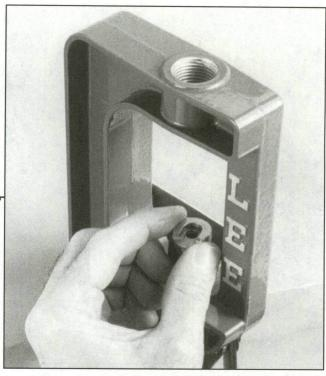
Step 3 - Installing the Shellholder: Choose the proper shellholder for the round you are loading. They usually come with the die sets. Raise the ram slightly to snap the shellholder into place with a twisting motion. Position it with the open side out to the left.
