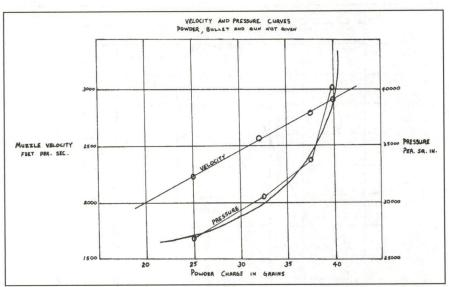
(Above) The pressure-velocity curve illustrates the relationship between velocity and the pressure generated by adding more powder. As powder is added, more of the energy of the expanding gas is worked against the chamber walls and the gas against itself. Additional powder added at the top end of a load generates little additional velocity but considerably more pressure.
