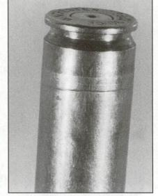
Excessive headspace signs begin as a backed-out primer. Stage two is the appearance of stretching and cracks. Stage three is separation. If excessive headspace is combined with an overload, stage three may be reached on the first loading.
