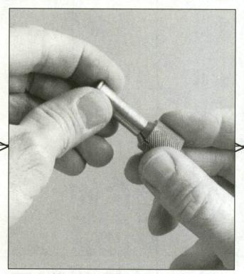
Step 6 - Chamfer and Deburr: To ease bullet entry, lightly chamfer the mouth of the case by inserting the pointed end of the chamfering/deburring tool into the case mouth and gently twisting it.
