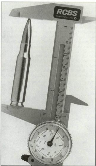
Finished cartridges should be checked to see they do not exceed overall length. If they do, the seater stem in the die can be adjusted to seat the bullets deeper.
