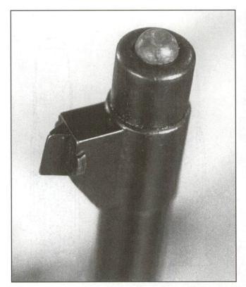
(Above and right) Slugging the bore consists of carefully driving a small, soft pure lead slug down the barrel. If done from both ends, the two slugs can be compared for tight and loose spots in the barrel.
