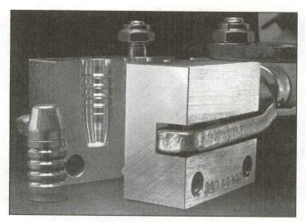
Aluminum moulds do not require as much breaking-in as iron or steel moulds. However, the cavity must often be coated with either carbon smoke or a special compound to get good bullets.
