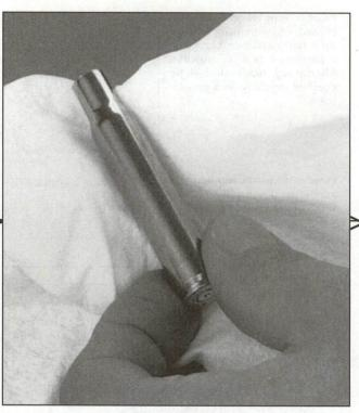
Step 1 - Clean and Inspect: It's always a good idea to wipe each case clean to prevent dirt from scratching the case and resizing die. Look for split necks, case cracks and anything else that would compromise safety. Destroy any defective cases by crushing, and then throw them away.
