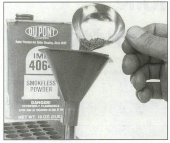
The reloader's powder funnel is especially designed to fit over the case mouth and deliver powder without spills. One size fits nearly all commonly reloaded cases.
