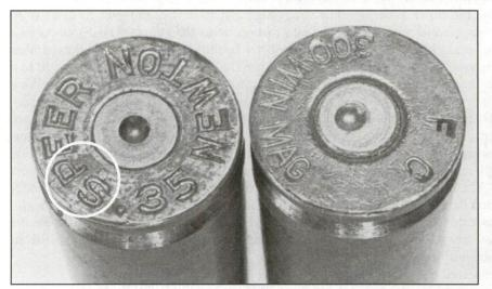
Was the flat primer on the left a result of high pressure or being too soft? The answer is likely high pressure since the case head also flowed into the extractor groove (circled).
