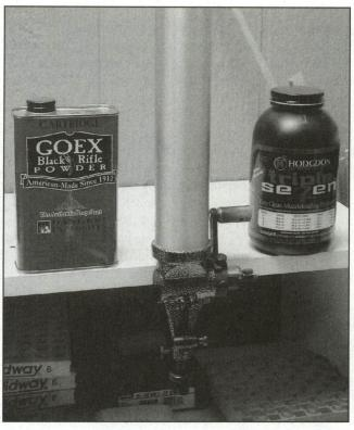
Lyman's #55 Blackpowder Measure is specially designed for use with blackpowder and blackpowder substitutes.
