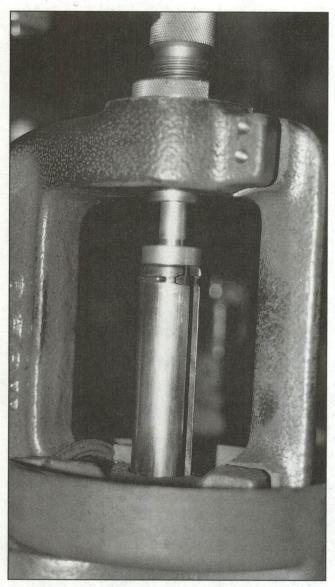
Partially sizing revolver brass will often allow a better fit in the chambers.
