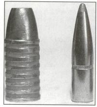
The cast/lubricated bullet will give equal or better accuracy than the jacketed hunting bullet, while producing less barrel wear, and can be made at a fraction of the cost. At ranges of 100-150 yards, it will kill just as effectively.
