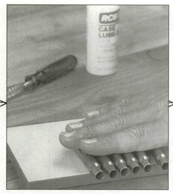
Step 2 - Lubricate the Cases: To prevent the case from sticking in the sizing die, it must be lubricated only with sizing die lube. With a bit of lube on the pad, roll a number of cases over it a few times to lightly coat the case body.
