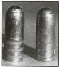
Bullets should be inspected before sizing and lubricating. Good cast bullets should have square edges and even grooves.
