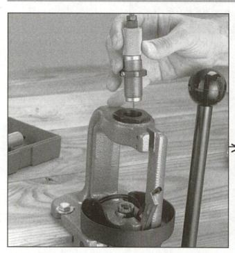
Step 4 - Adjusting the Sizer Die: With a shellholder installed in the ram, and the ram all the way up, thread the sizer die into the press until it touches the shellholder. Raise the press handle a little and turn the die in another 1/8- to 1/4-turn, then set the die lock ring.
