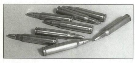
All are ready to shoot, except the one in the middle is a 222 Magnum and the rest are 223. If you plan to load similar calibers, extra caution is needed to keep the cases, loaded ammunition and, in some instances, bullets separate.
