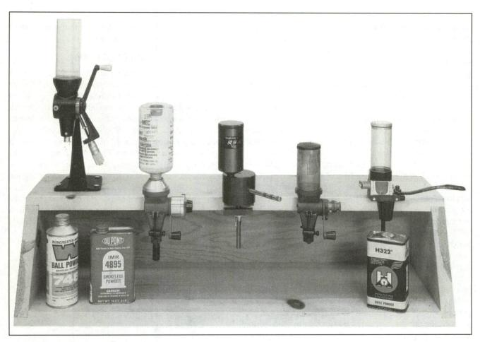
A powder measure speeds production and can throw accurate loads. Precision, however, depends on the consistency of operation.
