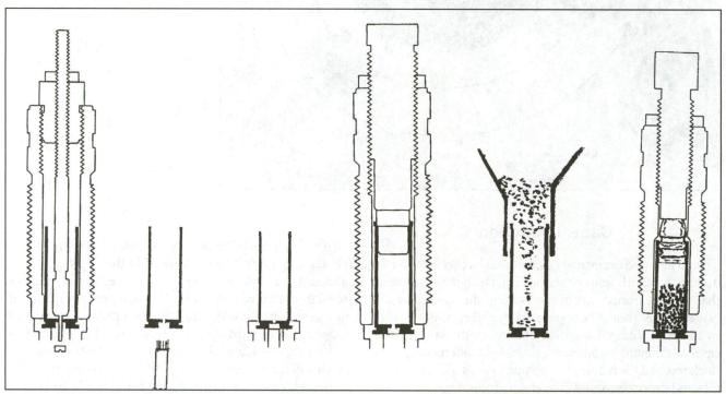
The basic steps in handgun reloading include: resizing and decapping, primer pocket cleaning, priming, case expanding, powder charging and bullet seating.
