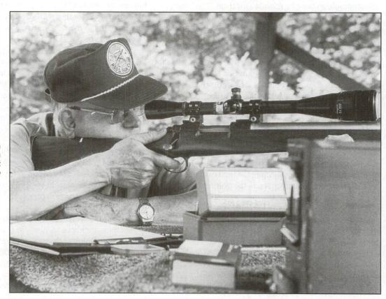
**Testing ammunition** should be done with a solid rest, firing at a known distance to determine accuracy.
