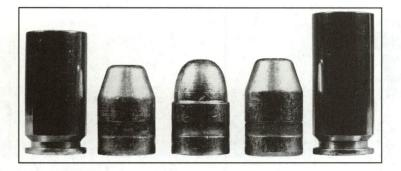
The 40 S&W with (from left): the 180-grain FP, 185-grain RN, and 200-grain FP bullets, and a 10mm Auto case on right.
