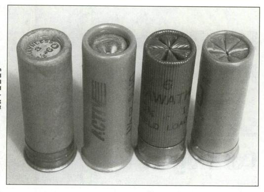
Various crimp styles, from left: an old-style rolled crimp on a paper shell with top wad; the rolled crimp, still used and necessary for making slug loads; typical six-point and eight-point crimps.
