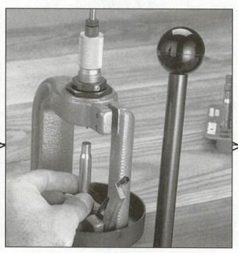
Step 5 - Case Resizing: Insert an empty case into the shellholder and gently lower the press handle all the way to the bottom, running the case into the sizing die. Doing so will resize the case to factory dimensions and knock out the fired primer. Raising the press handle will lower the case and expand the case mouth to the proper dimension to hold the new bullet.
