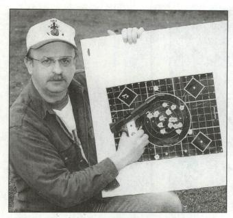
What is accuracy? Here, author shows a 25-vard target into which he fired 200-grain factory loads on a test of the ammunition's performance in his customized Auto Ordnance 45 pistol. But author has found that his groups can tighten up when he stokes magazines with handloads using 230-grain Speer TMJ bullets over a charge of HP-38.
