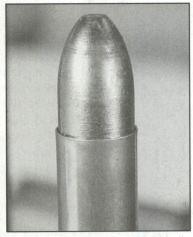
Bullet fully seated to the predetermined depth and ready for crimping in a separate operation.
