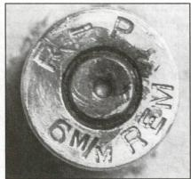
A leak around a primer indicates an expanded primer pocket. Time to discard the case.
