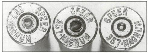
The cratered primer (center) appears at first glance to be evidence of excessive pressure. The actual cause was an oversize firing pin hole and a soft primer.
