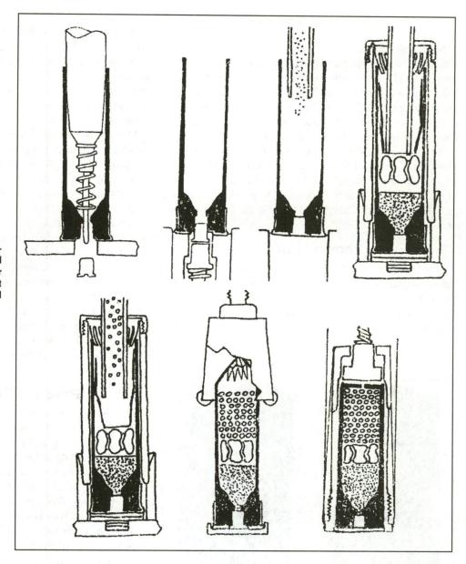
There are seven steps in shotshell reloading: resizing and decapping, priming, powder charging, wad seating, shot metering, crimp starting and crimp finishing.
