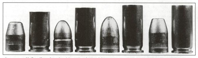
9mm cases and bullets. Shown here (from left): a 122-grain FP and the 9mm Luger; a 125-grain RN and the 9x21; a 145-grain RN and the 9x23 Winchester.
