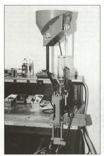
Dillon XL 650 with automatic case feeder. All you have to do is put in a bullet and pull the handle.
