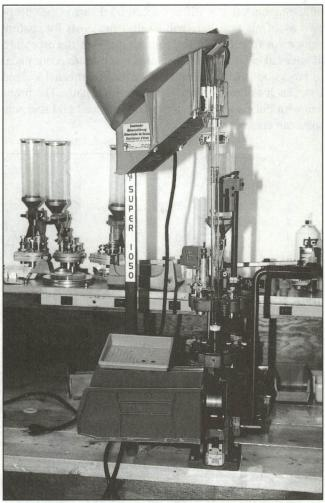
Top of the line Dillon 1050 can load around 1000 rounds per hour.
