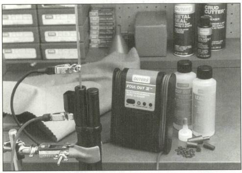
Outer's Foul Out III electrochemical system is the easiest method of dealing with serious metal fouling problems.
