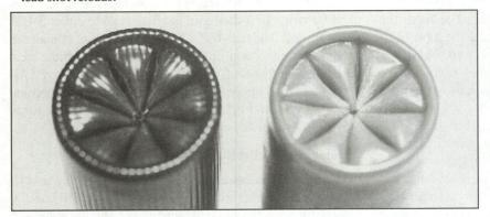
Steel reloads require good quality crimps with firm closures to provide the resistance necessary to insure good combustion from the slower burning propellants used in steel reloading.
