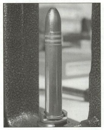
45-70 with the bullet seated approximately half-way to the final depth.
