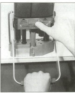
Step 3 - Powder Charging: Slip the shell into the wad guide at Station 3, lower the handle and slide the charge bar to the right to add the powder.
