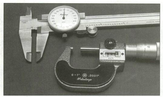
A micrometer and/or precision caliper capable of accurate measurement to .001-inch are necessary tools. Investing in good-quality equipment is worthwhile in the long run.
