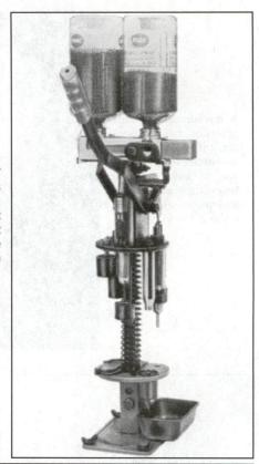
move a shell from one station to the next, even a basic machine like the Lee Load-All II will turn out 100 rounds per hour. Lee offers update kits to convert older presses to the Load-All II and conversion kits to load other gauges. Hornady offers a similar single-stage press and a conversion to progressive loader status via a kit. The MEC 600 Jr. Mark V, while a single-stage machine, is set up for speed and will double the Lee's output.
