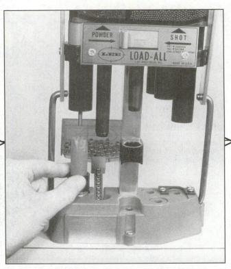
Step 1 - Sizing: Sort your hulls by brand and type, and discard the defective ones. Slip the sizing die, grooved end up, over the shell. Place the shell in Station 1 and pull down the handle. This full-length resizes and deprimes the shell.
