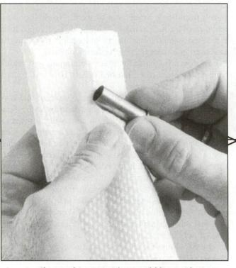
Step 1 - Clean and Inspect: It's a good idea to wipe cases clean before beginning to reload them. This also allows you to inspect them for any split necks, cracks, etc. Discard those that are damaged.
