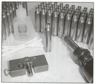
Case necks are turned so that wall thickness is consistent throughout its circumference. Variations of only .0001-inch are achievable with care. An expansion mandrel that fits the turner's mandrel precisely should be used. Many shooters turn the necks more than once with a series of turners to achieve the level of consistency they require. A K&M turner is shown. Many competitors use the Nielson turner for 6PPC and other small cases.
