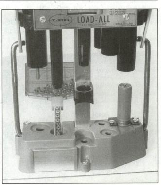
Step 7 - Final Crimp: Immediately move the shell into the shellholder at Station 5, and pull the press handle down to complete the crimp. That completes the loading cycle, giving you a readyto-shoot shotshell.
