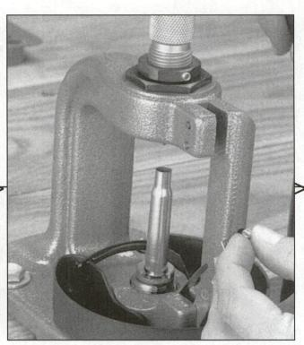
Step 9 - Priming (A): Place a fresh primer, anvil side up, into the cup of the primer arm and insert a case into the shellholder.
