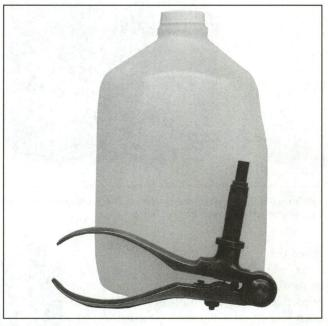
The Lyman #310 Tool is used to de-prime blackpowder cases which are then dropped into a gallon jug of soapy water to begin the cleaning process.
