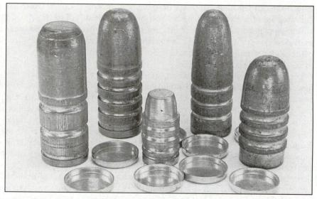
Copper gas checks applied to bullets designed for them will allow increased velocities and keep hot gas from melting the bullet bases.
