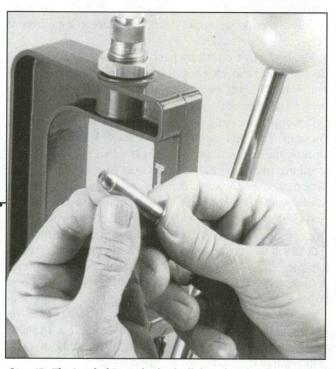
Step 15 - The Loaded Round: That's all there is to loading a handgun cartridge. A final wipe with a clean cloth and the ammunition is ready to be fired. Don't forget to mark the ammo box with your load data so you can repeat the load.
