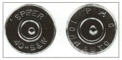
Even though the 40 S&W and the 10mm Auto have the same case and bullet diameters, they use different size primers.
