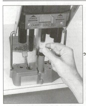
Step 4 - Inserting the Wad: Raise the handle, insert the proper wad and lower the press handle until it stops.
