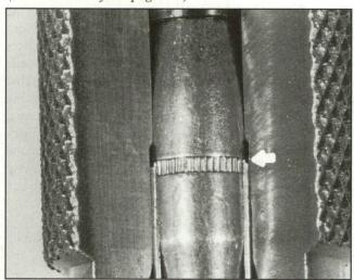
Seating dies have a crimping shoulder in them to crimp some hunting bullets. Never crimp bullets that do not have a crimping cannelure in them.
