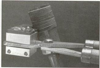
Never hit the sprue cutter with anything made of metal. A wooden dowel, in this case wrapped with rawhide, makes an effective cut without damage to the mould.
