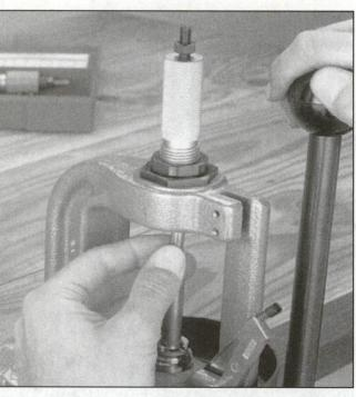
Step 17 - Bullet Seating (C): With the handle up, insert a primed and charged case in the shellholder, and hold a bullet over the case mouth with one hand while you lower the press handle with the other, easing the bullet and case up into the die. This will seat the bullet. Measure the loaded round to see if the bullet is seated deeply enough.
