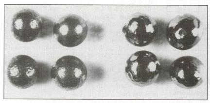
Besides being rounder and more uniform, steel pellets differ from lead shot in other important ways. Steel pellets (left) are much harder and less compressible. These characteristics significantly change the ballistics of steel versus lead loads, requiring the use of different wads and powders than when reloading lead.
