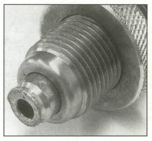
Problems such as crimped-in primers and stuck cases, like this one with the head torn off, require special tools such as a stuck-case removal kit.
