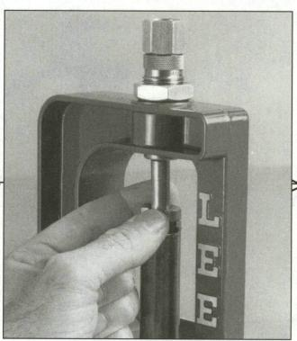
Step 7 - Case Mouth Expansion: After installing and properly adjusting the expander die, insert a case and run it into the die to bell the case mouth for easy insertion of a new bullet. Adjust the die just enough to allow easy bullet entry.
