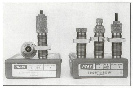
Reloading dies come in two basic formats-a two-die set for rifle cartridges and a three-die set for pistol and cast-bullet rifle loading.
