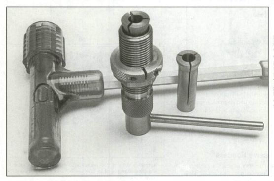
Bullet pullers come in two varieties: those that mount on the reloading press and those of the hammer-type kinetic variety (left). The latter is perhaps gentler on bullets, but requires more energy on the part of the user.
