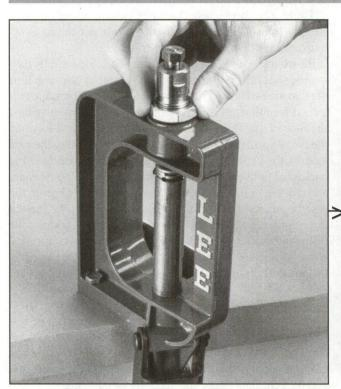
Step 4 - Adjusting the Sizer Die: Raise the ram to the top of its travel and screw the sizing die in until it just touches the shellholder. Now, slightly lower the ram and screw in the die an additional 1/4-turn. Tighten the lock nut.
