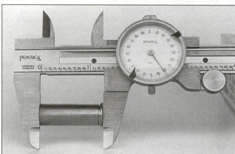
Case length should be checked after sizing and neck expanding, because the case stretches in these operations.
