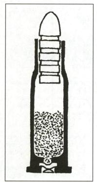
Never seat a cast bullet below the bottom of the neck into the shoulder area of a bottleneck case. The base will be melted and expanded, ruining accuracy and raising pressure.
