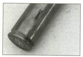
Case failures are not common, but they do happen. The nearer to the case head the rupture, the more serious it is.
