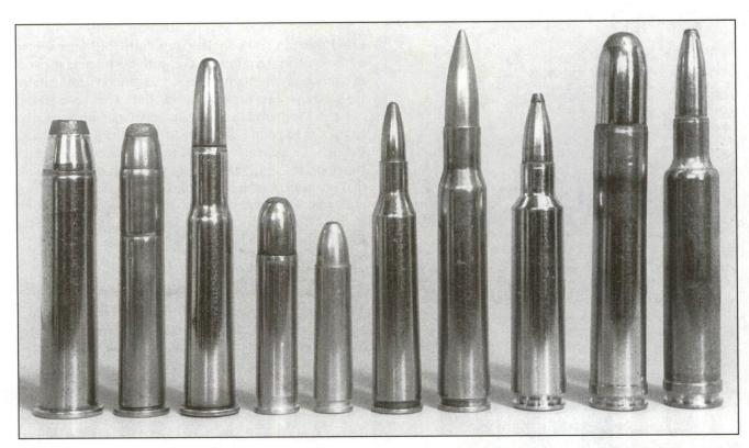
(Above) Basic cartridge case forms include the following variations, left to right: straight-walled rimmed (45-70), straight-tapered (38-55), rimmed bottleneck (30-40 Krag), semi-rimmed straight (35 Winchester SL), rimless straight (30 Carbine), semi-rimmed bottleneck (220 Swift), rimless bottleneck (30-06), rebated head (284 Winchester), straight belted (458 Winchester Magnum) and bottleneck belted (7mm Weatherby Magnum).
