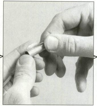
Step 2 - Lubricate the Cases: Case lube is needed when not using a carbide resizing die. Spread just a light film on each case with the fingers.
