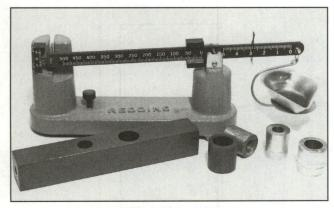
The most important tool for any steel shot reloader is a good scale. It should be used to adjust powder and shot bars or bushings to throw within the tight limits demanded by steel. Then it should be used frequently during the reloading process to check actual powder and shot charges being dropped.
