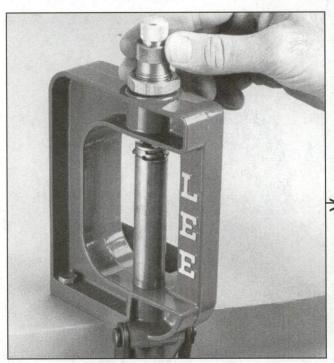
Step 12 - Bullet Seating (A): To install the bullet-seating die, place a case in the shellholder and raise the ram to the top of the stroke. Screw in the seater die until you feel it touch the case mouth. If no crimp is desired, back the die out 1/2-turn. If you want a crimp, turn it in 1/4-turn.
