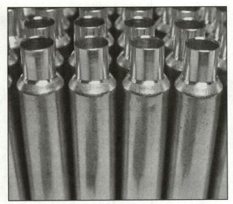
Continuing the cut into the shoulder approximately .03-inch to .04-inch helps prevent a doughnut from forming in the neck. The cut forms a small lip at its end. When the case is fired, that lip is forced to the inside of the case as the brass molds itself to the configuration of the chamber. When the lip moves inside and travels forward into the neck, an irregular venturi is formed that can presumably affect velocity and pressure differentially.
