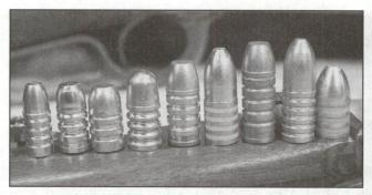
Blackpowder hunting bullets should have a flat point or large round nose with many grooves for carrying lots of lube. Shown are bullets in 38-, 40-, 45-, & 50-caliber from bullet moulds by Lyman, RCBS, SAECO, and custom mould maker Steve Brooks.
