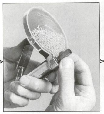
Step 8 - Priming: Installing a new primer can be done on the press or with a hand-held Auto Prime tool. After filling the primer tray, slip a deprimed case into the shellholder and press the lever to push a primer into the primer pocket. Follow the instructions that come with each tool.
