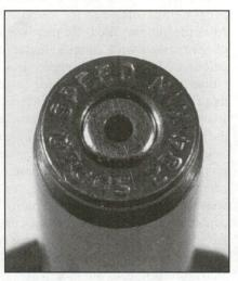
A pierced or "blown" primer can be caused by excessive pressure or a firing pin that is too long or too sharp. (Photo courtesy Speer.)
