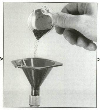
Step 10 - Powder Charging (B): Lee's expander die allows the powder charge to be dumped from the scale pan into the primed case through the die. Cases can also be set into a loading block for powder charging.
