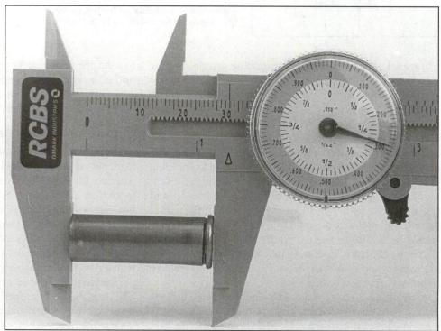
Finished ammunition should be measured to see that the cartridge does not exceed the maximum overall length specified in the loading manual.
