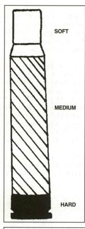
(Left) The modern brass cartridge is made hard and thick where the greatest amount of support is needed, springy in the body for easy extraction, and soft at the mouth to ensure a good gas-tight seal when fired.
