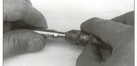
(Above and left) A deburring tool makes bullet seating easier and lessens damage to the bullet base.
