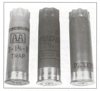
While steel shot can be reloaded in the same hulls used for reloading lead, the increased capacity of hulls such as the Federal Gold Medal plastic hull (center) are the best for reloading steel.
