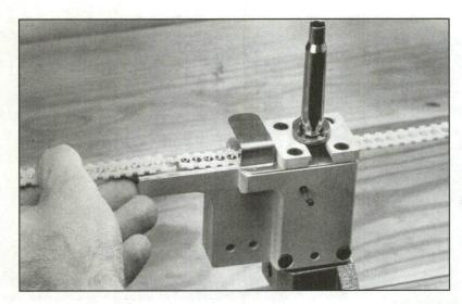
The RCBS APS primer feeder uses plastic strips instead of the conventional stacking tube, reducing the hazard of sympathetic detonation. (Photo courtesy RCBS.)
