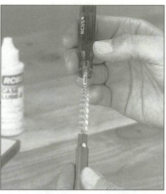
Step 3 - Case Neck Lubrication: Use a case neck brush to clean and lubricate the inside of the case neck. This will reduce resizing effort and neck stretching. Only a small amount of lube should be applied to the brush.
