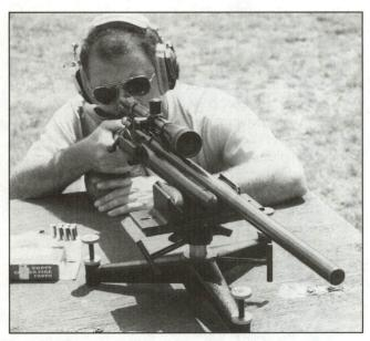
Author bench testing a Krag-actioned 219 Zipper. For those unfamiliar with the cartridge, it performs on a par with the 223 Remington but operates at lower chamber pressure due to the larger case size. Scope is a Lyman 6x silhouette model.
