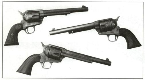
The circa-1879 44-40 Frontier Six-Shooter (center) is to be used only with blackpowder or blackpowder substitutes. It is joined by a 3rd Colt Single Action and a Cimarron Model P artificially antiqued to represent the same time period.
