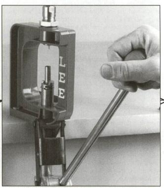
Step 5 - Case Resizing: Place a lubed case in the shellholder and raise the ram, guiding the case as it enters the sizing die. This step also knocks out the fired primer. Raise the press handle and remove the case.
