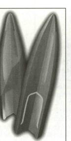
Nosler's Partition and Combined Technology Partition Gold bullets are designed so the front half expands in conventional manner, but only to the center. A heavy partition keeps the back half intact, retaining weight and energy, while an ordinary bullet might fragment.
