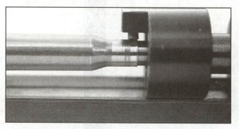
Functioning as a miniature lathe, the Forster tool can be adjusted to remove a minute amount of brass from a case neck. The cutter, that small cylindrical piece that bears against the case neck, is raised or lowered by means of Allen screws and subsequently locked in place.
