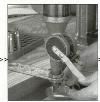
Step 14 - Powder Charging (C): Another method of charging is to use the powder measure. It dispenses a precise, uniform charge with each crank of the handle, thereby speeding up the process. Use the reloading scale to adjust the powder measure until it throws several identical charges. Then, weigh about every ten charges to recheck the weight.
