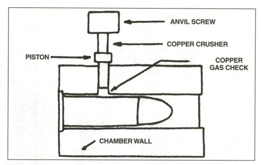
This is a drawing of a simplified crusher-type pressure gun used for measuring pressure. Pure copper and lead slugs are compressed to determine peak pressures on firing.
