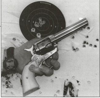
Don't think a single-action revolver with fixed sights is accurate enough? Here's a 15-yard target author fired using handloads charged with H-110 and 100-grain Speer JHPs.
