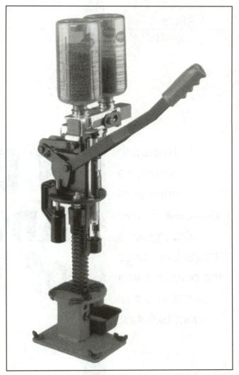
The MEC 600 Jr. Mark V can turn out an average of 200 rounds per hour. It's available in 10, 12, 16, 20 and 28 gauges.
