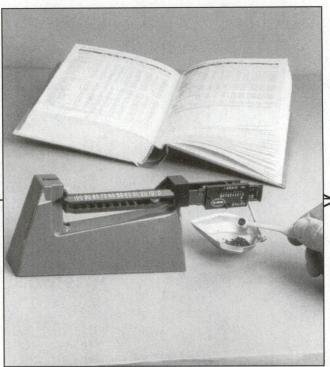
Step 9 - Powder Charging (A): Find the proper and safe load for your cartridge in a loading manual or from another reliable source, then weigh each charge on your powder scale. This is the safest method, although a bit slow, and is best for accuracy and maximum loads.
