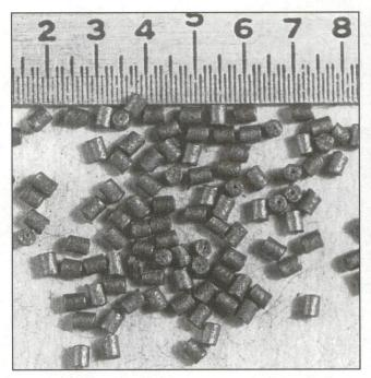
IMR 4320 is a slow-burning single-base rifle powder for use in large-bore and high-powered rifles. The extruded grains are of a "short cut" size.
