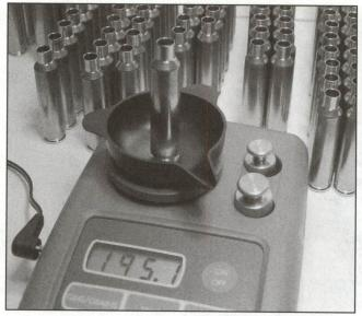
Cases are meticulously weighed and separated, particularly in long-range benchrest events. Identical case dimensions and weight are necessary to control velocity and pressure variation. Large velocity spreads produce non-competitive vertical dispersion. Modern digital scales speed up the process. They are capable of AC or DC power, are small and easily packed, and can be used outdoors with the use of a clear plastic box. The readout is clear and not easily confused.
