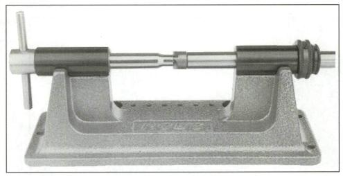
outside diameters, case neck wall thickness, checks for bullet roundness and diameter, case swelling, etc.
