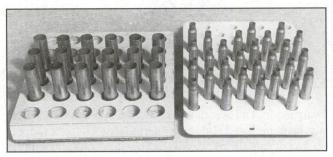
Loading blocks can be homemade from wood (*left*) or of moulded plastic (*right*). Loading blocks are not merely a convenience; they are a necessity to keep you from double-charging a cartridge case.
