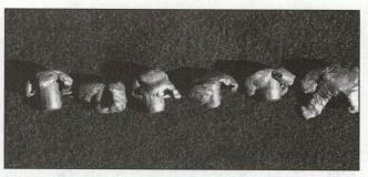
A group of 30-caliber 180-grain bullets recovered from big game. With each bullet, major bones were hit and adequate penetration realized at ranges from 75 – 250 yards. These are what well-constructed bullets should look like.
