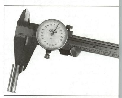
Sorting brass by neck thickness helps ensure the bullet be well-centered in the case and crimping more uniform.
