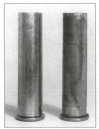
Low pressure is evidenced by the soot stains on the case on the right, which failed to make a complete gas seal when fired.
