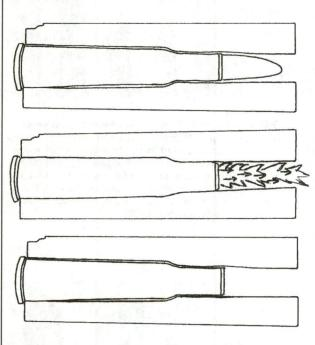
to load, those that went into breech-loading guns still had not solved the breechloader's basic problem of gas leaks. Many attempts were made to deal with the early breechloader's nasty habit of spewing fire and smoke out of the joint between breechblock and barrel into the face of the shooter. The actions also tended to stick and eventually jam when they became encrusted with blackpowder fouling. It was
