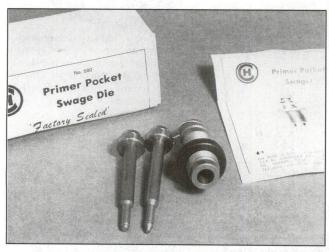
Primer crimps are easily removed with this handy tool (and others), which also swages the primer pockets to uniform size.
