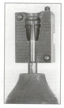
nose of the bullet. The theory behind these is that they give a more perfect base, since base regularity is the most important factor in accuracy with cast bullets. Nose-pour moulds are generally custom-made and intended for long-range, heavy target bullets.
