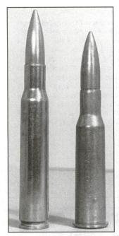
The U.S. standard 30-06 Springfield cartridge (left) and Russian 7.62x54mm Mosin rifle cartridge are not compatible. Some Russian rifles have had chambers recut to take the '06. The smaller-diameter 30-06 has plenty of room to swell and burst in the oversize Russian chamber.
