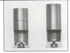
The balloon-head case on the 38 Special at left offers more powder capacity, and thus lower pressure. However, this is a weaker design than the solid-head 357 Magnum case on the right.
