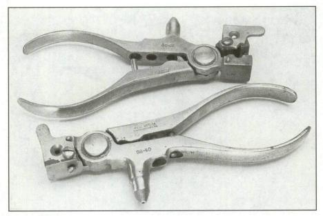
(Below) The Lee Hand Press Kit is a modern version of the old Ideal tong tool. The kit includes dies, case lube, powder dipper, etc.
