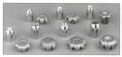
These Speer Gold Dot handgun bullets in 38, 40 and 45 calibers evidence considerable expansion after being fired into ballistic gelatin.
