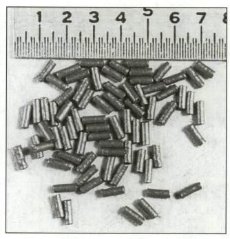
IMR 3031 powder is an extruded single-base propellant made of nitrocellulose. It has a fairly slow burning rate and has long been a standard for military rifle cartridges.
