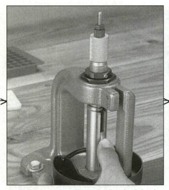
Step 10 - Priming (B): Lower the press handle and push the primer arm all the way into the slot in the ram.
