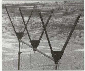
The plastic parts can be considered expendable items. They are inexpensive to replace should damage occur. Pictured are the Oehler 35P skyscreens, diffusers, rail, and rail stands.
