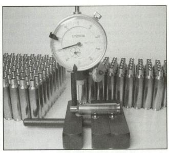
Case concentricity is checked to insure that the case will be axially aligned with the chamber. Check the body as well as the neck and a seated bullet. Do so prior to sizing, with a bullet seated, and again after firing. If the loaded and/or unloaded cartridge is not concentric, this procedure will allow the reloader to determine whether the sizing die or the chamber is at fault.
